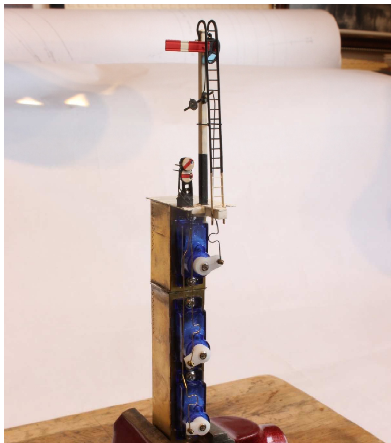
LNWR timber post with 5' arm for inner home plus LMS twin discs controlling access to sidings.
