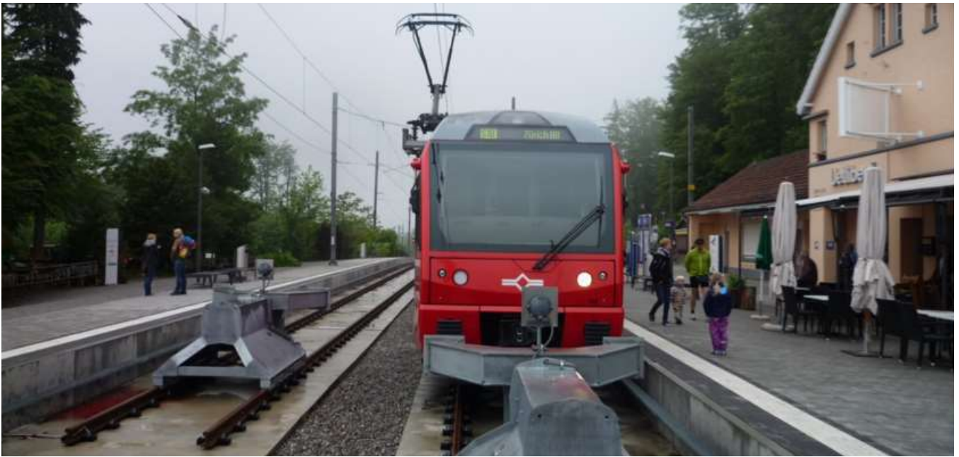
A Stadler Be510 EMU at Uetliberg station. The offset catenary and pantograph can be clearly seen in this view.
