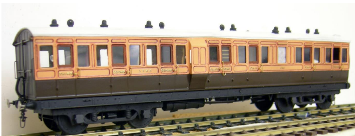
LSWR 48ft Brake Tri-composite coach. Built 1891. The additional length had provided a guard's compartment, and once again only first class passengers have use of a toilet
