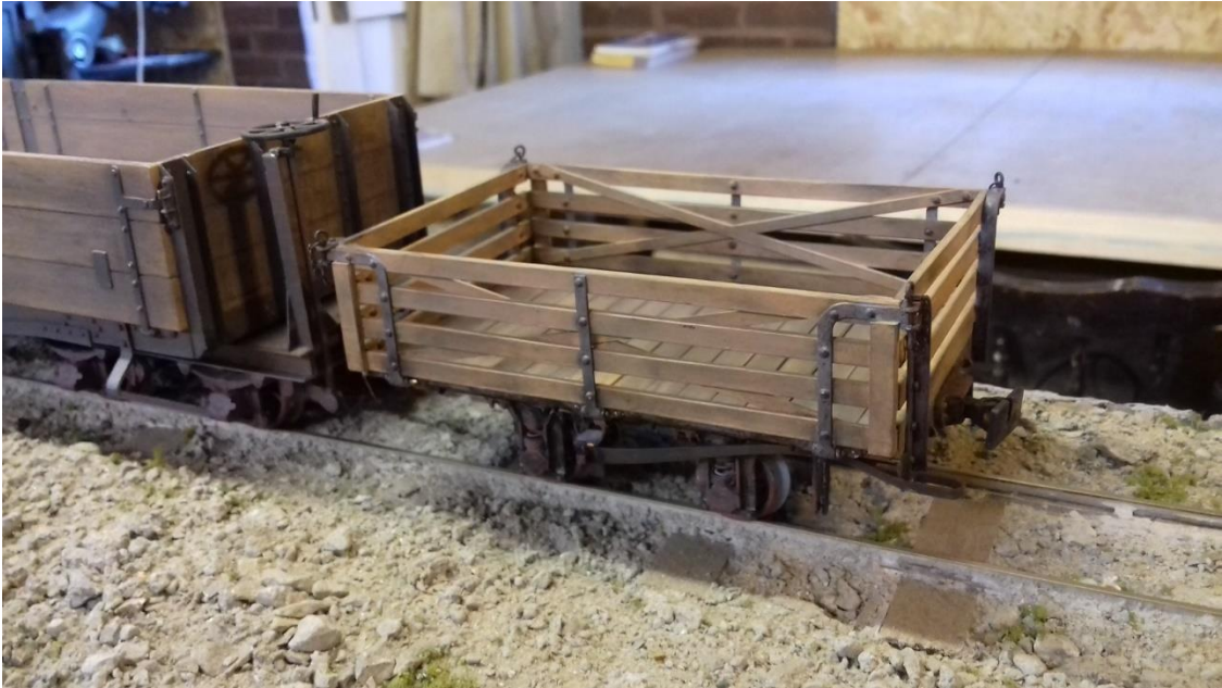
A Severn Models WDLR ration wagon built from one of Andrew Vaughan's etched brass kits. It is 16mm to the foot scale narrow gauge running on 32mm track.
