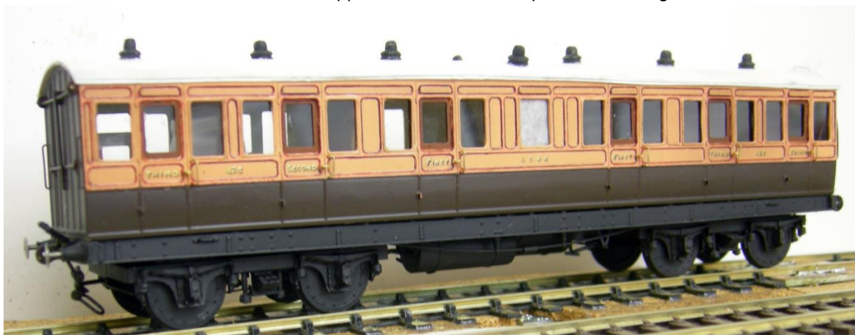
LSWR 42ft 6in Tri-composite coach. Built 1889. The lavatory could only be accessed by the first class passengers.
