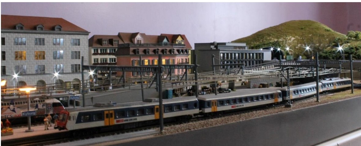
An RBDe560 “Colibri” EMU approaches Kyburg with a local St Gallen to Zurich train. The 4-car Colibri units are widely used on local services on the SBB (the Swiss Federal Railway). My model comprises four hand-made bodies mounted on three Marklin coach chassis and an American Z-Lines (AZL) motorised “Bud” chassis. The latter uses a coreless motor and runs beautifully.
